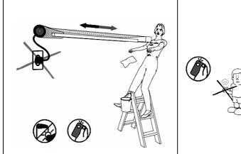
$\triangle$  When working in the range of travel (e.g. cleaning and maintenance work), it is to be ensured, that the awning is switched de-energized (e.g. switch off safety device, disconnect plug coupling on the motor cable, ...) There is a risk of being crushed and falling down.
