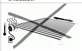
3. Extending and retracting the awning several times in quick succession causes the automatic shutdown of the motor, which is thereby protected from overheating. After cooling down, the motor automatically switches back to standby.
