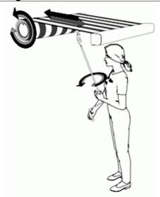
Attention: In party extended position and with flat pitch angles (less than 14'), there is an increased risk of water collecting on the surface of the cover. The optimal cover tension is with the awning extended.
