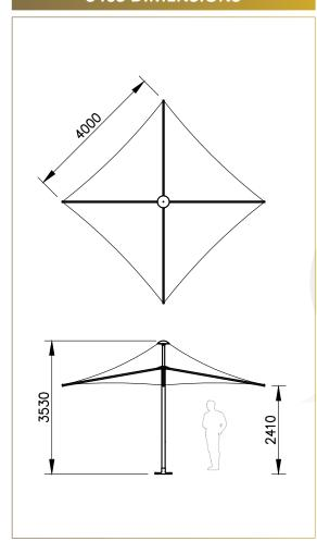
The brilliance of our Sunset umbrellas is that in extreme weather conditions they can be retracted easily and quickly. The unique gearing mechanism neatly concealed within the column of the umbrella allows the unit to be wound down via removable handle or automatically via remote control, ideal for cafes, restaurants and holiday resorts.
