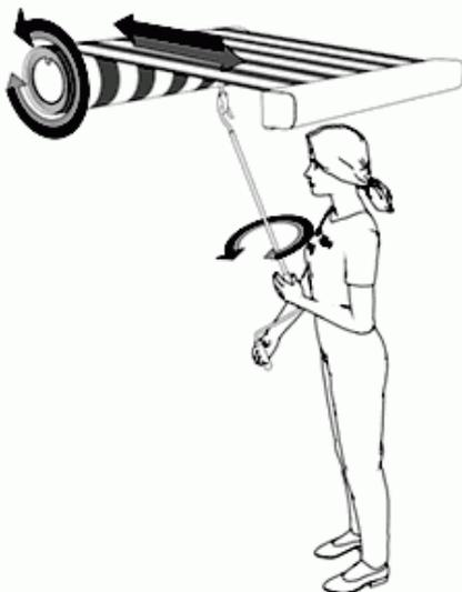
**3.1** Engage the hook of the crank rod in the transmission eyelet.
